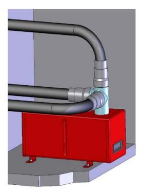
3-Way Manifolds can also be used to install three separate tubing branch lines.
