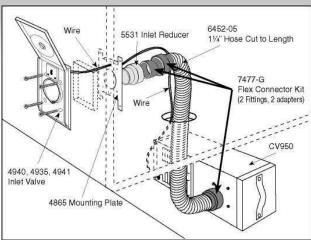
Above picture and illustration show installation using two hose adapters and only one spigot fitting from the Flex Kit.
