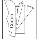
Once the fabric has reached its full extension, grasp pull straps and attach them to the pull strap catches. 052869-004
