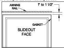
SLIDEOUT CLOSING AND SEALING WHEN IT IS IN THE COMPLETE RETRACTED POSITION.
