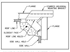
room. CAUTION: MAKE SURE THE BRACKETS ARE ALIGNED SO THE SCREWS WILL BE GOING INTO THE SIDEWALL AND THE ROOFLINE OF THE SLIDEOUT ROOM. THIS IS NECESSARY TO ACHIEVE PROPER SUPPORT. BRACKETS THAT ARE ATTACHED TO ONLY A THIN METAL OR FIBERGLASS SKIN WILL NOT SUPPORT THE TORQUE THE SIDEOUT KOVER GENERATES!
