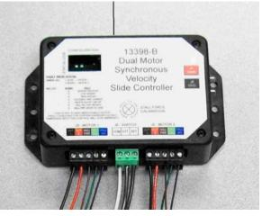
3. The room may now be pushed in or out as desired. Larger rooms may need several people to push. Try to keep both sides of the room even. When the room is completely in, plug both motors back in to the controller, this applies a brake to the motors and keeps the room locked in position.
