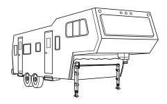
The landing legs of a 5th wheel trailer are used for positioning the trailer during hookup and unhooking from the tow vehicle and as support during camping and stowage. They level the trailer to allow the refrigerator to operate properly and to provide comfort for the users. They are not designed to be the sole support for the weight of the trailer during tire changes or servicing.
