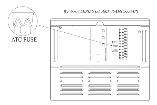
If fuse(s) are blown this means the RV Battery was accidentally connected in reverse either at the battery or at the converter. Connect properly then replace the fuse(s).
