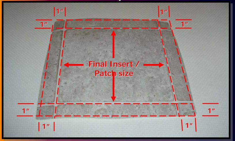
Cut an insert piece that is at least 1" inch larger on each side than the material being replaced.
